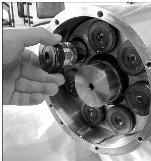
7. It is recommended to place the pistons upside down on an even clean base/surface.
