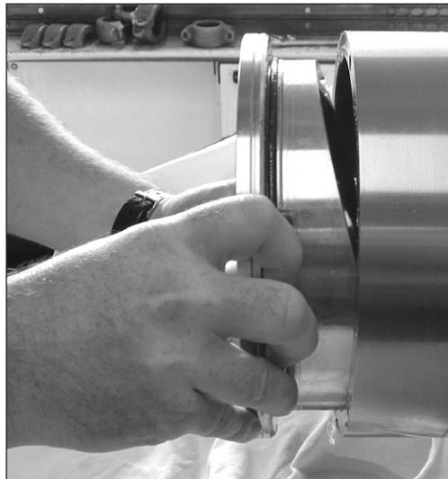
5. Place the swash plate upside down to avoid scratches on the surface.
