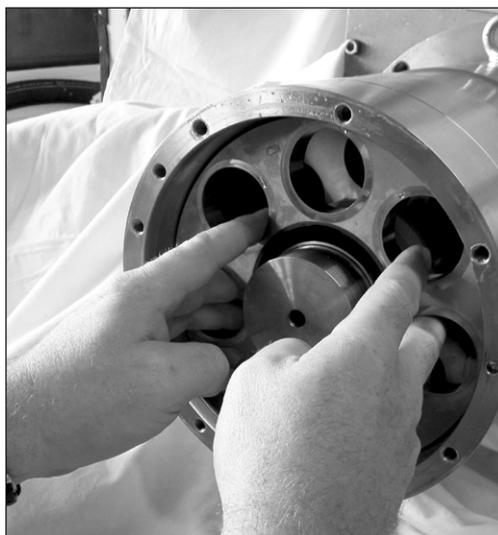
2. Ensure that the retainer plate is oriented correctly with its slant surfaces pointing downwards.
