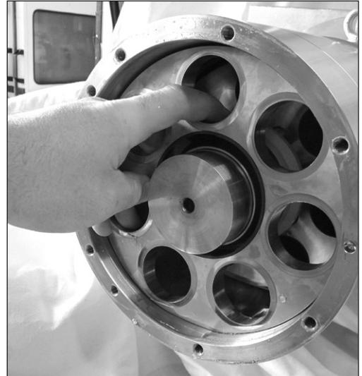
9. Inspect the piston bushings in the cylinder barrel for scratches or other damages. Small scratches are accepted if there are no hard particles in the bushings.
