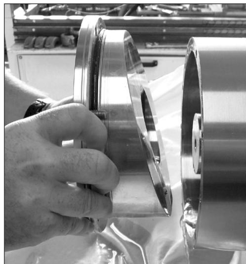
6. Mount the 3 screws as shown below. Turn each screw a couple of rounds at the time, to ensure the swash plate is pulled as straight forward as possible.
