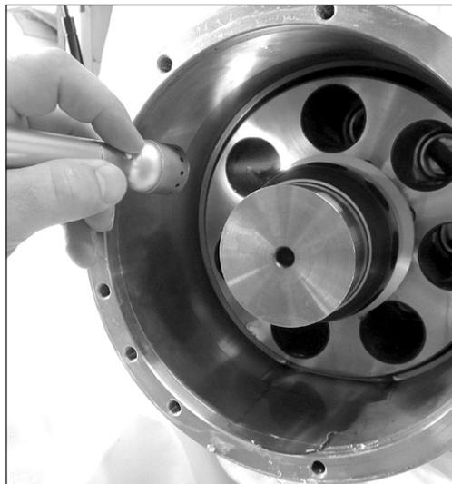
10. If any worn pistons are found, all pistons must be replaced. See page 7.
