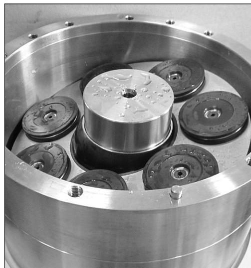
4. Replace the O-ring on the mounting flange.
